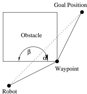
Fig. 7. Example obstructed path and waypoint selection.
