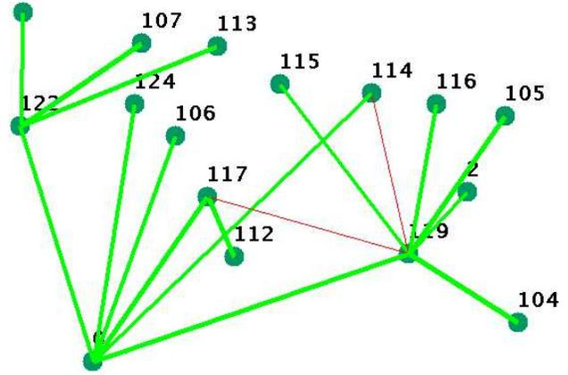
Fig. 16. Multihop network topology created by TinyDB.
