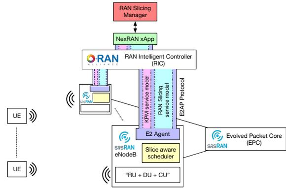
Figure 1: NexRAN Open RAN open source RAN slicing
