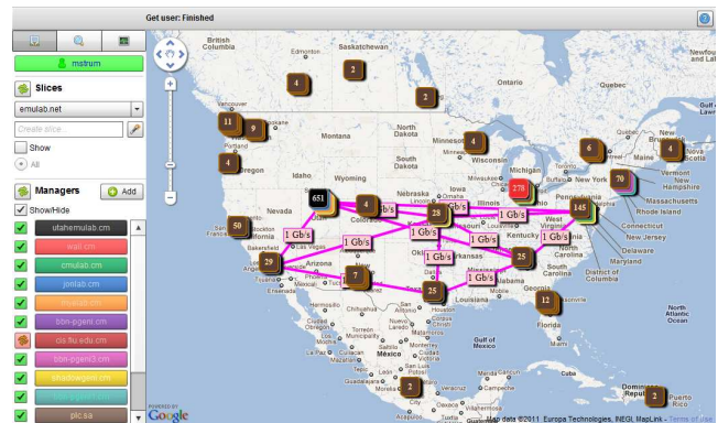
Figure 1: Screenshot of Flack, showing the map view of resources on the right, and a list of the user’s slices and GENI’s aggregate managers on the left.
