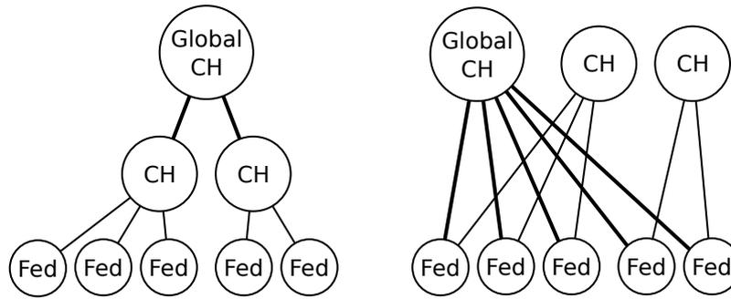
**Fig. 3** An inter-federation consists of one clearinghouse for the entire inter-federation (“Global CH”), one clearinghouse per federation (“CH”), and a potentially large number of individual federates (“Fed”). The structure on the left illustrates a single root of trust per federation (see Section 4.1), while the flatter arrangement on the right shows multiple roots of trust per federation (Section 4.2).
