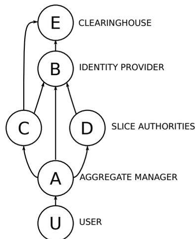
**Fig. 1** An example of entities interacting within a federation. The principals are described in Sections 1.1 and 2; the arrows indicate trust relationships, described in Section 3.
