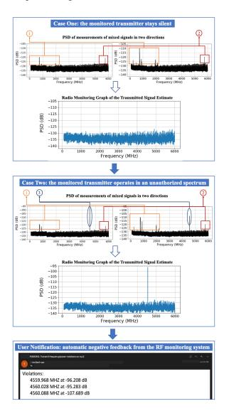
Figure 2: BITSS Workflow: ① incident signals from the environment; ② incident signals from a known external source; ③ transmitted signal at an unauthorized frequency.
