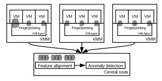
Figure 1: Fluorescence architecture.
