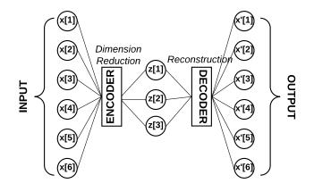
Figure 2: Autoencoder architecture.
