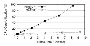
Figure 6: Protection against Heartbleed vulnerability: DPI-based vs. eZTrust.
