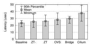
**Figure 4: Fast path packet latency.** "Baseline" indicates server-to-server latency. "ZT" and "ZT-" refer to eZTrust with and without policy rules, respectively.
