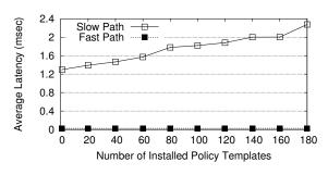
Figure 3: Latency: slow path vs. fast path.
