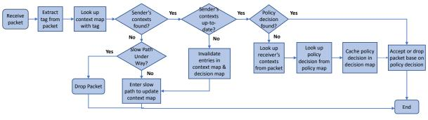
Figure 2: eVerifier's packet verification procedure.
