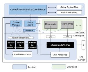
Figure 1: The eZTrust architecture.
