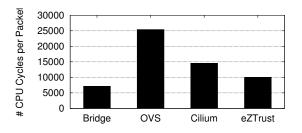
Figure 5: Per-packet CPU usage for policy processing.
