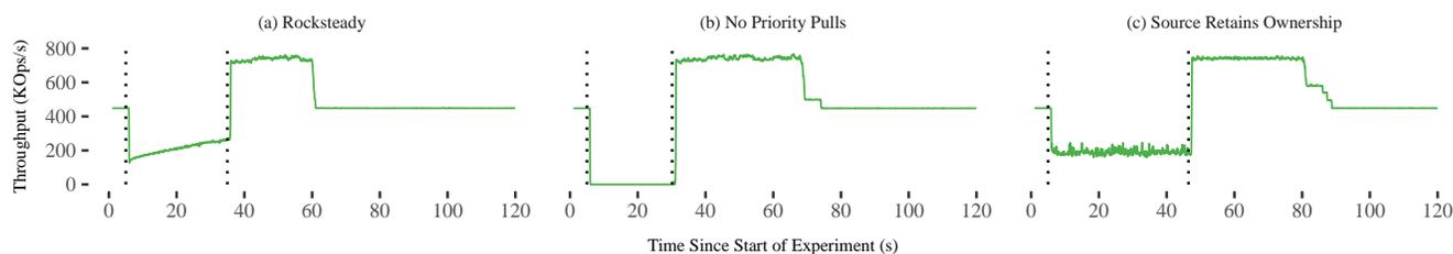
**Figure 9: Running total YCSB-B throughput for (a) Rocksteady, (b) Rocksteady with no PriorityPulls, and (c) when ownership is left at the source throughout the migration. Dotted lines demarcate migration start and end.**
