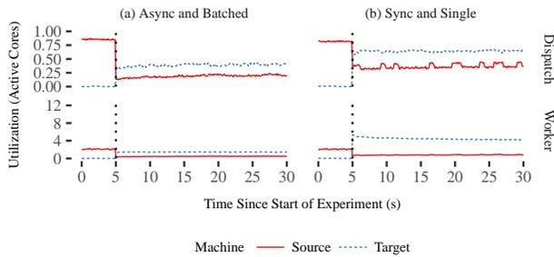
**Figure 14: CPU Load with no background Pulls. Asynchronous batched PriorityPulls improve dispatch and worker utilization at both the source and target compared to synchronous Pulls that stall target worker cores.**
