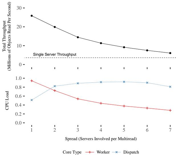
**Figure 3: Throughput and CPU load impact of access locality.** When multiget always fetch data from a single server (Spread 1) throughput is high and worker cores operate in parallel. When each multiget must fetch keys from many machines (Spread 7) throughput suffers as each server becomes bottlenecked on dispatching requests.
