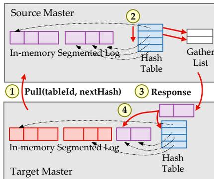
**Figure 6: Overview of Rocksteady Pulls.** A Pull RPC issued by the target iterates down a portion of the source’s hash table and returns a batch of records. This batch is then logically replayed by the target into its in-memory log and hash table.
