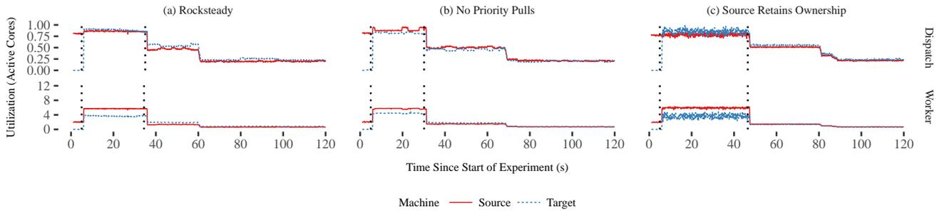
**Figure 11: Dispatch core and worker core utilization on both source and target for (a) Rocksteady, (b) Rocksteady with no PriorityPulls, and (c) when ownership is left at the source throughout the migration.**
