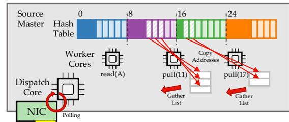
**Figure 7: Source pull handling.** Pulls work concurrently over disjoint regions of the source's hash table, avoiding synchronization, and return a fixed amount of data (20 KB, for example) to the target. Any worker core can service a Pull on any region, and all cores prioritize normal case requests over Pulls.
