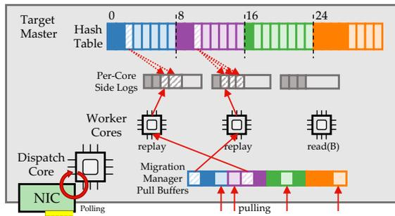
**Figure 8: Target pull management and replay.** There is one Pull outstanding per source partition. Pulled records are replayed at lower priority than normal requests. Each worker places records into a separate side log to avoid contention. Any worker core can service a replay on any partition.
