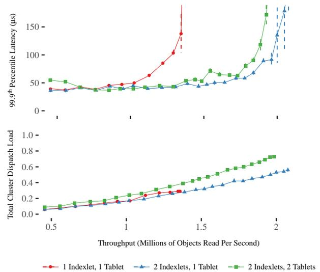
**Figure 4: Index scaling as a function of read throughput.** Points represent the median over 5 runs, bars show standard error. Spreading the backing table across two servers increases total dispatch load and the 99.9<sup>th</sup> percentile access latency for a given throughput when compared to leaving it on a single server.
