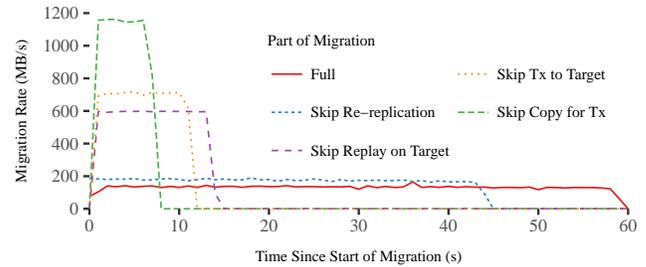
**Figure 5: Bottlenecks using log replay for migration. Target side bottlenecks include logical replay and re-replication. Copying records into staging buffers at the source has a significant impact on migration rate.**
