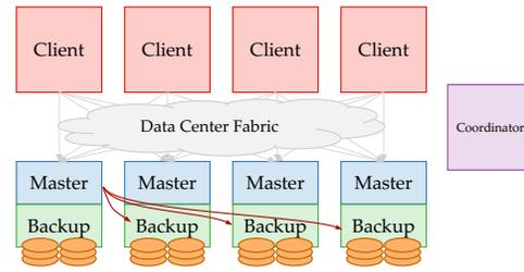
**Figure 1: The RAMCloud architecture.** Clients issue remote operations to RAMCloud storage servers. Each server contains a master and a backup. The master component exports the DRAM of the server as a large key-value store. The backup accepts updates from other masters and records state on disk used for recovering crashed masters. A central coordinator manages the server pool and maps data to masters.
