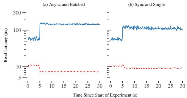
**Figure 13: Median (dashed line) and 99.9<sup>th</sup> percentile (solid line) access latency without background Pulls. Async batched PriorityPulls restore median latency almost immediately compared to sync PriorityPulls.**
