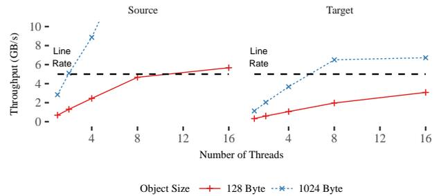
**Figure 15: Source and target parallel migration scalability. Source side pull logic can process small 128 B objects at 5.7 GB/s. Target side replay logic can process small 128 B objects at 3 GB/s. For larger objects, neither side limits migration.**
