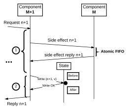
Figure 14: ECHO's components operate atomically and in client's FIFO order.
