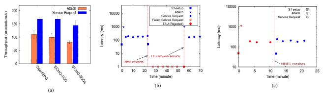
Figure 12: (a) Throughput of Attach and Service Request; (b) Unmodified OpenEPC MME crash results in an outage; (c) ECHO MME crash avoids outages.
