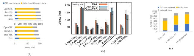
Figure 10: Latency overhead of ECHO: (a) Attach (top) and Service Request (bottom) procedures latency on 1DC deployment, observed on eNodeB; (b) Latency of each individual message in an Attach (left part) and Service Request (right part) procedures on 1DC deployment; (c) Latency for attach procedure on 1DC and 3DC deployments.
