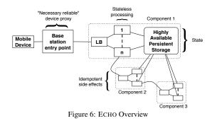
ation. ECHO moves the main components of EPC into the cloud, replicating them for reliability while connectivity to the UEs is through the base stations which implement our entry point serialization. Existing public cloud load-balancers provide load-balanced connectivity to the "regular" Internet and to the Internet-based access "backhaul" between base stations and the public cloud.
