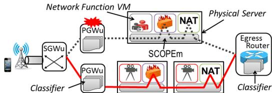
Figure 7: Service-Chain routing in SCOPE.
