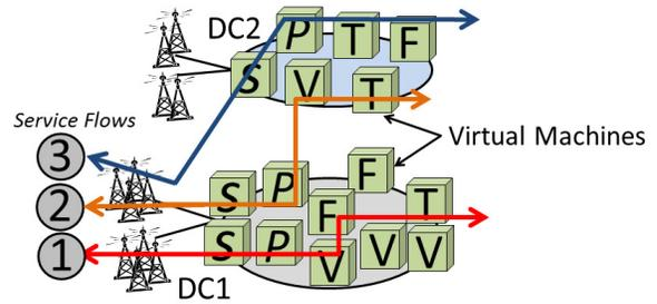
Figure 3: Service Flow allocation in SCOPE.
