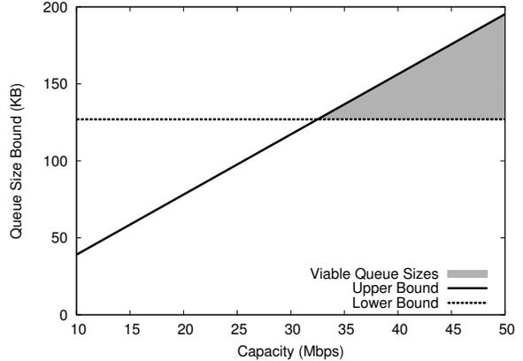
Figure 1: The relationship between capacity and the bounds on queue size for a path with  $ABW_f = ABW_r = 10$  Mbps,  $RTT_{base} = 20$  ms, and  $w_{max} = 65$  KB. Low capacities prevent any viable queue size.
